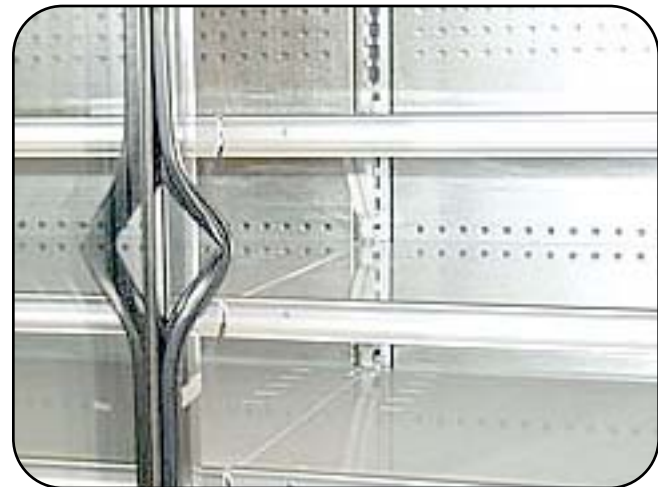
Figure 11. Improperly Installed or Damaged Gasket
